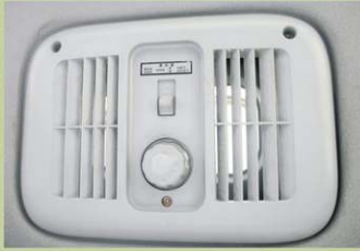
Roof Ventilator for air Ventilation.
