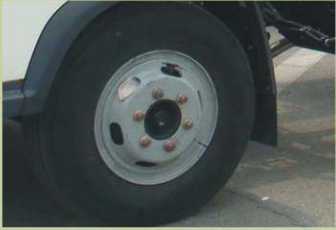
Radial tyres of 7.50-16 and stud-piloted 06-hole steel disc .
